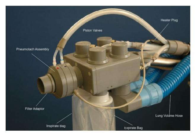
NOTE: Two different valve designs exist. Key differences are detailed below in the instructions.
